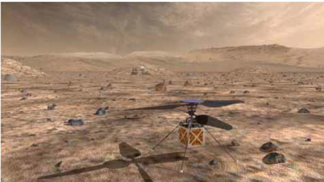
A proposed helicopter could triple the distances that Mars rovers can drive in a Martian day and help pinpoint interesting targets for study.
